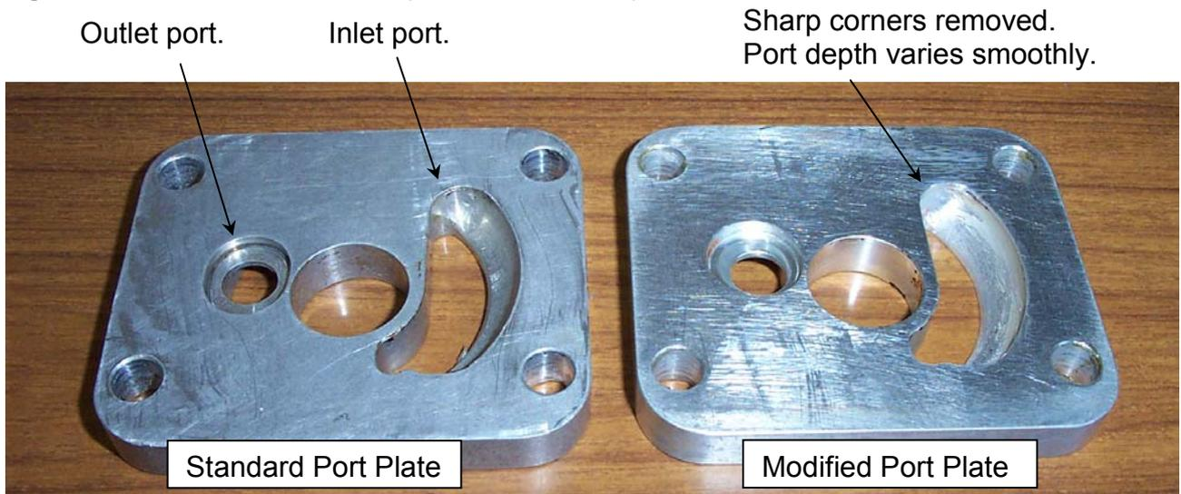
**Figure 2. Rear Side of Port Plates (Tractor Installation)**
