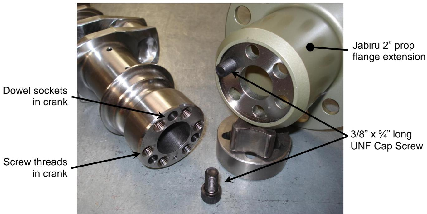
Figure 1 – Flange & Crankshaft
