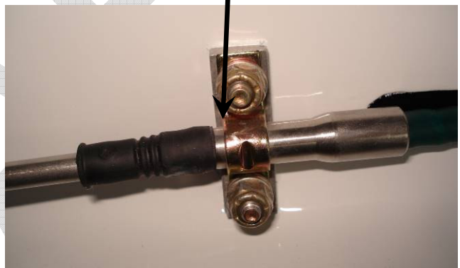
Figure 2 – Clamp Comparison & Installation (Rudder Cable)
