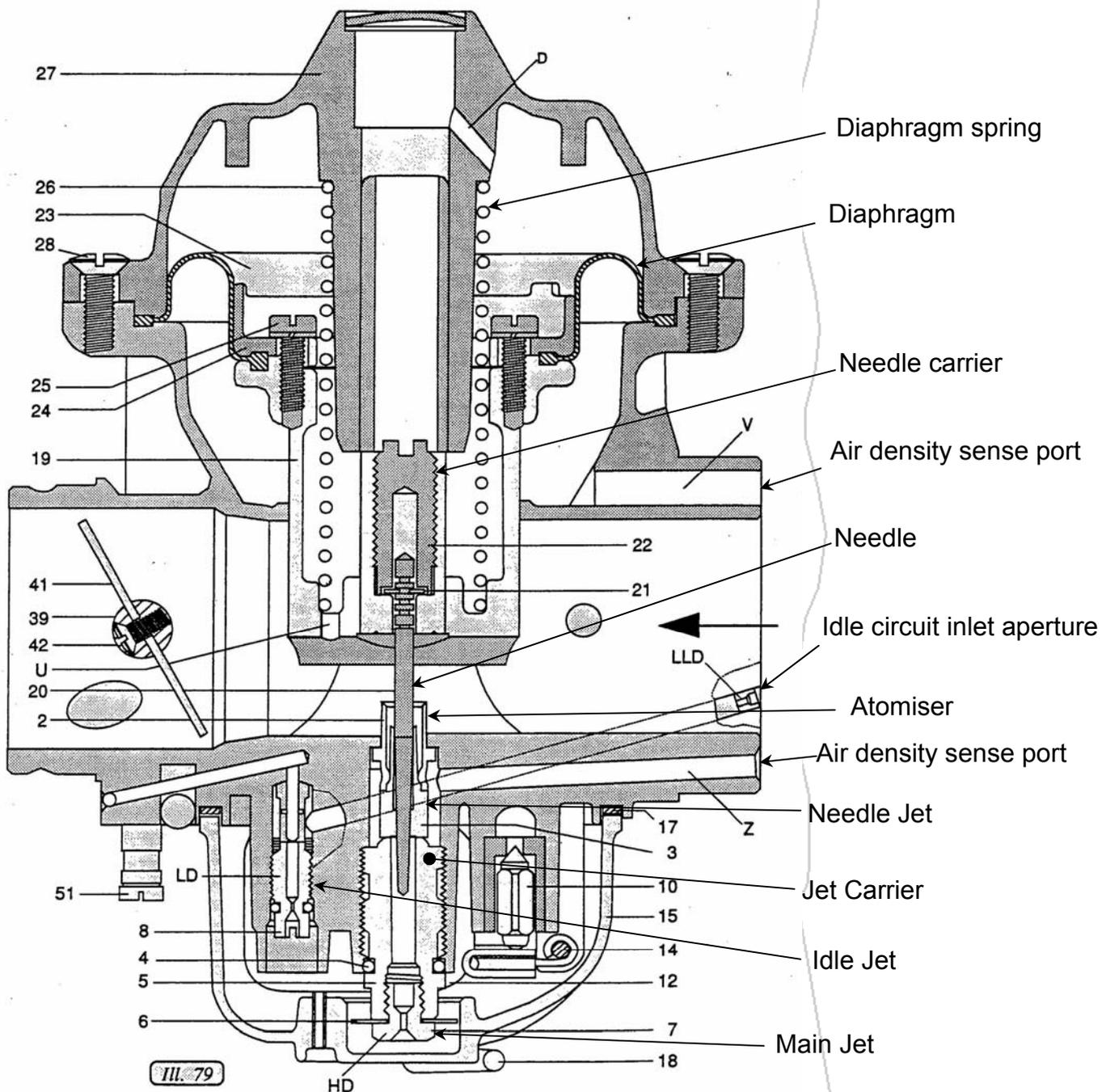
Figure 1. Carburettor Cut Away Drawing
