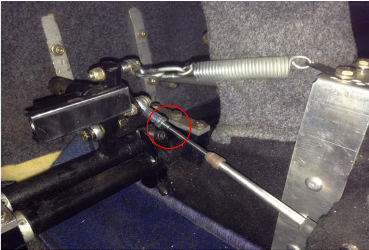
Figure 1 – Location where cable broke.
