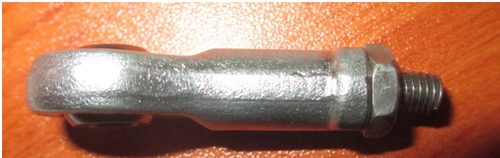
Figure 2: Rod end with broken end of cable.
